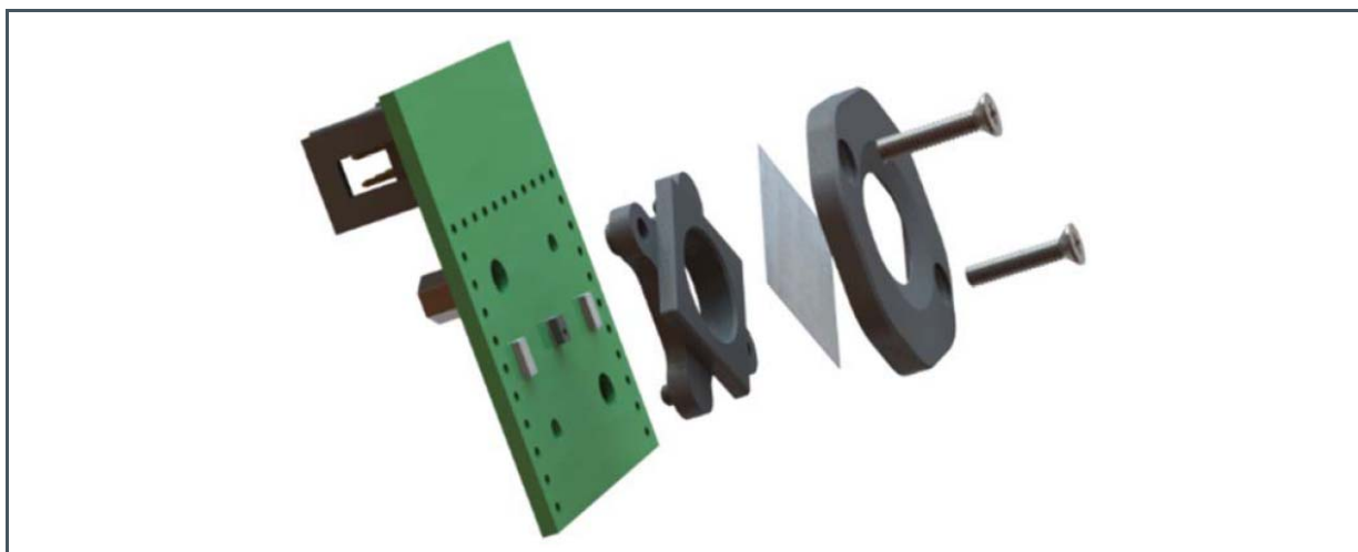
Figure 6: Installation of Diffusor Holder on AS7343 EVK
